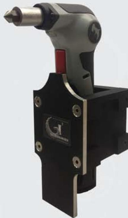
The device can break multiple windows on a single charge. There are NO electrical connections needed between the tool and the robot. Simply pick up the tool and push it up against the window you intend to break. This device only requires 2 lbs. of force to activate, making it ideal for smaller robotic platforms.
